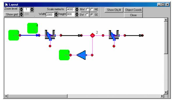
The act of shrinking or expanding conduits on the layout does not change the actual underlying design dimensions. The lengths of the pipes and channels in your design will remain as you specified in the use of the Route command. The layout image is a conceptual representation of the drainage network.
