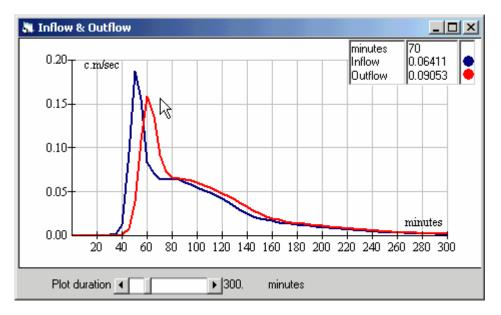
Note the peak is reduced from 0.188 c.m/s to 0.158 c.m/s and lagged by about 10 minutes. Since the hydrographs are plotted at 5 minute increments, very 'peaky' hydrographs may sometimes show some truncation of the outflow.
